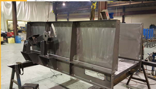
Conveyor Section with Custom Metering Wheel
