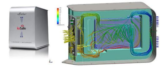
Using SOLIDWORKS Flow Simulation software, ioSafe optimized the balance of air flow for cooling and outward steam flow during a fire.
