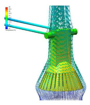
Figure 8: Particle tracks over the lamp, mounted horizontally and facing downwards, showing how the natural convection causes the air to flow smoothly over the exterior of the lamp housing. The thermal plume contracts as the flow accelerates above the lamp.
