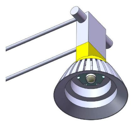
Figure 5: The 3D CAD representation of the LED luminaire SOLIDWORKS Flow Simulation automatically models any internal cavities as fluid regions, a requirement for analysis. While the need for this step is more obvious for a pipe carrying a liquid, it is also necessary to predict the air flow through and around the luminaire.
