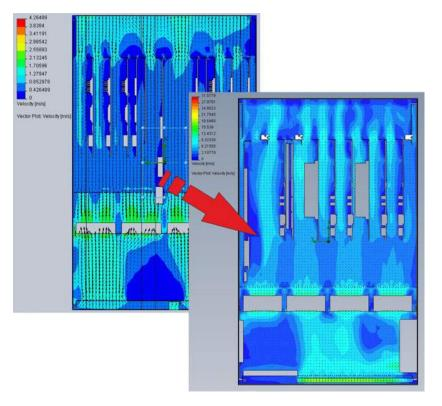
POLYRACK uses SOLIDWORKS Flow Simulation to optimize designs for racked electronic systems, producing betterperforming designs without the need for extensive and expensive prototypes
