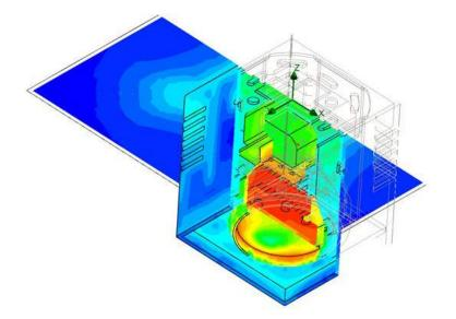
Figure 3: Temperature inside an LED lamp shown with a 50 percent slice.
