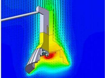
Figure 7: Temperatures on a 2D slice through the center of the lamp with vectors showing flow caused by natural convection over the outside of the lamp.
