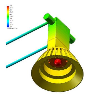
Figure 9: Predicted surface temperatures shown on the 3D CAD model
