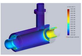
Temperature distribution (fluid and solid) in SOLIDWORKS Flow Simulation
